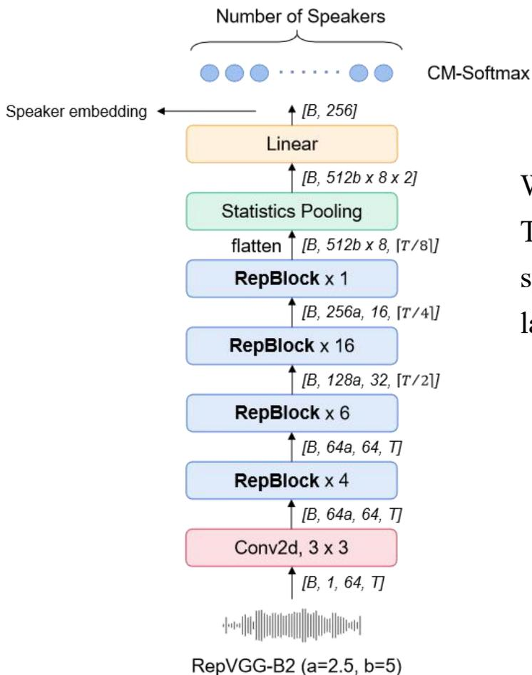
We used ResNet, RepVGG, ECAPA-TDNN in our system. Take individual system RepVGG as an example, our system is composed of backbone, pooling, embedding layers and loss function.
